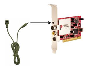
Now fasten the other end of the receiver cable to your monitor or the housing of your computer by using the adhesive strip included in the delivery quantity.
