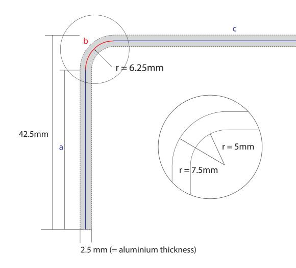
If you bend metal the center line (ideal assumption) remains the same length, whereas the outer line is stretched and the inner line is compressed.
